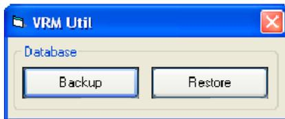
2. After the mouse icon changes from the hourglass to the standard pointer, you can close the program. It will have created a file in the same directory called **vrn.bak**. This file is the backup of the database structure and information. You need to copy this file to the workstation you wish to migrate to for the VRM install. It must be placed in the same directory as the VRMUtil.exe program.
