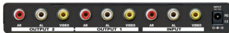
Rear View : Audio/Video Input : 1x Composite Video/Stereo Audio Audio/Video Output: 2x Composite Video/Stereo Audio Power input : DC+12V, @300mA
